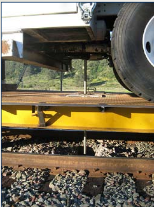
Photo 2: Close-up of cone through low-railer
