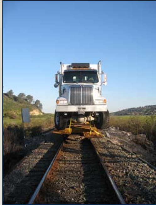
Photo 1: CPT rig positioned on low railer
