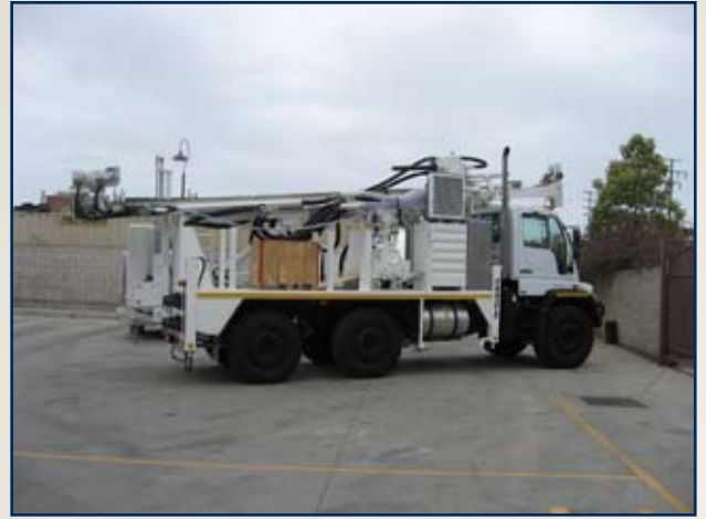
Pitcher Drilling's new 6 x 4 Mud Rotary Drill Rig
