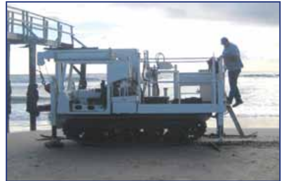
14 Ton track mounted CPT rig is suited for off road areas with rugged terrain.
