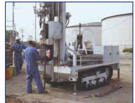
The Marl M5T (above) and 1.5T rig (below) can be used in locations requiring limited access and low overhead clearance.
