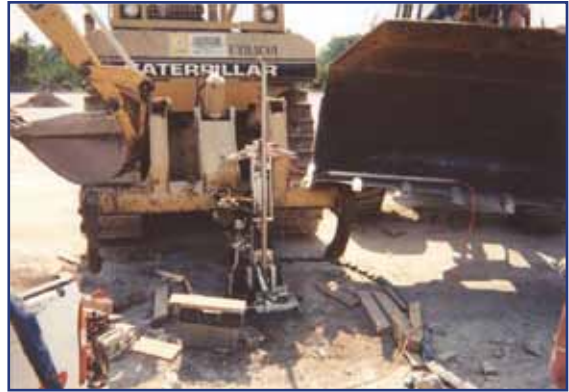
CPT Portable Ramset Mounted on Dozer Ripper Assembly - Guatemala
