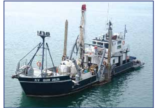
The Quin Delta drill ship is best suited for offshore foundation and liquefaction studies, soil sampling and coring, and for establishing baseline conditions and determining material quantities for dredging programs.
