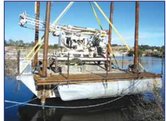
Portable spud barge developed for water 3' to 20' in depth and capable of anchoring in deeper waters.
