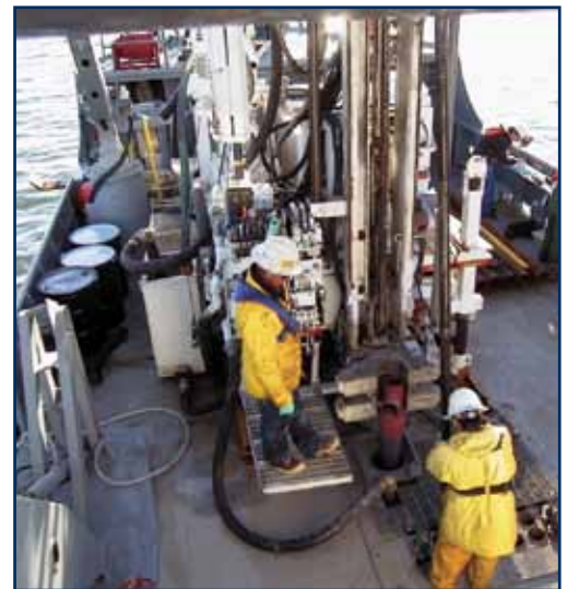
Mobile B-80/22 marine drill rig can be used for sampling or sediment and rock coring.
