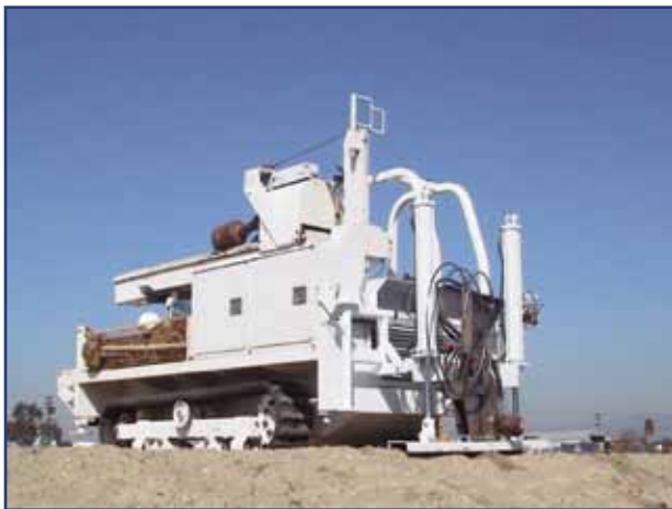
Mini CPT system can accompany direct push and all terrain equipment for use on land.
