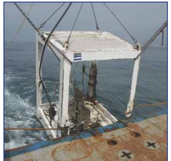
The Mini CPT ready for deployment in self-righting seabed deployment frame which is lowered to the sea floor with a winch line.
