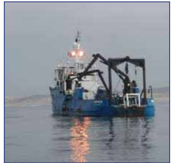
The Mini CPT can be deployed off the back of a ship using a simple A-frame and winch.
