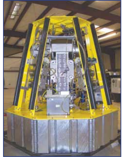
20 ton push capacity Seabed CPT unit
