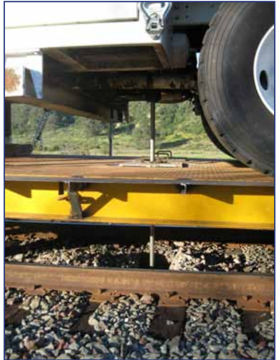
Conducting CPT through T-railer®
