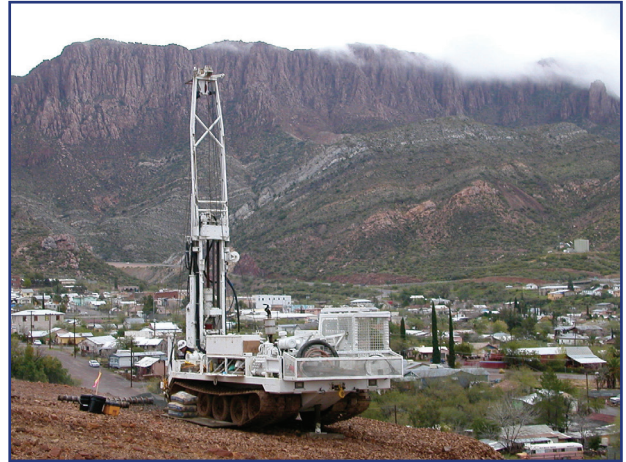
Designed for difficult access locations, the CME 850 is able to climb a 60% grade and transverse a 40% grade. The low pressure steel D-dent tracks allow less than 5psi pressure.
