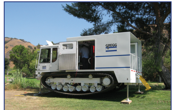
20 Ton track mounted CPT rig is suited for off road areas with rugged terrain.
