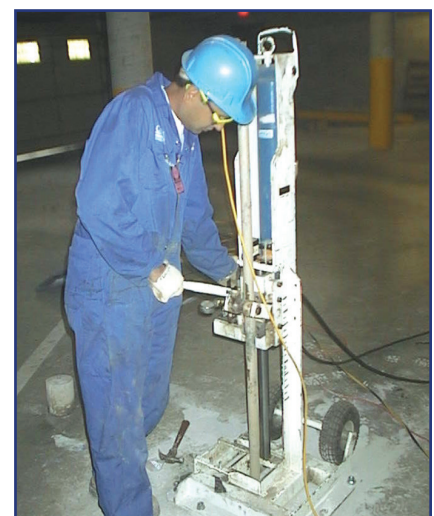
Ramset limited access CPT system requires only 5 feet of vertical clearance and has a footprint of only 2 square feet.
