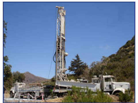
The Speed Star 30K is capable of drilling 1000+ feet and installing wells to 500+ feet. With 30,000 lbs of pull back and a casing hammer, this rig drills efficiently through rock deposits.
