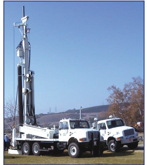
Versa Drill V100 can be used for soil liquefaction & environmental investigations and well installations.
