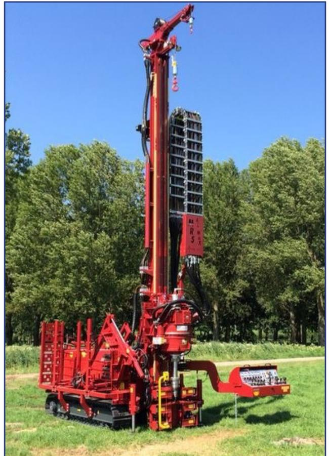
The Mid-Roto Sonic 50K features a full sized sonic drill head but a compact track mounted body for a smaller footprint on-site.
