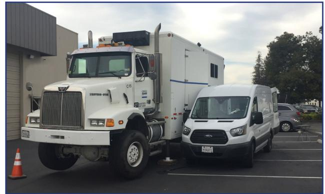
Gregg's CPT truck can be positioned next to the MIP control van for tandem operation.
