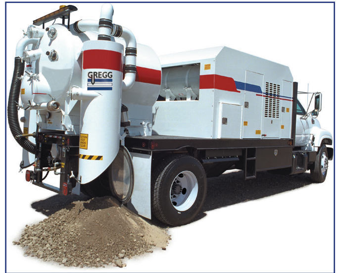
The air excavation system utilizes kinetic energy in a high velocity air stream to penetrate, expand, and break up soil.
