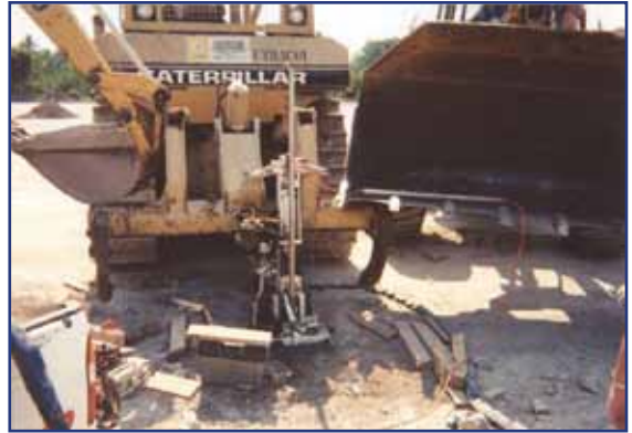
CPT Portable Ramset Mounted on Dozer Ripper Assembly - Guatemala
