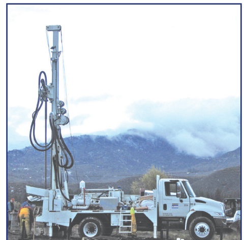
The Fraste MD/XU is a top head drive rotary rig with make up/break up clamps also capable of rock coring.
