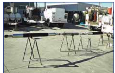
A straddle packer assembly is used to isolate pumping zones in a test well
