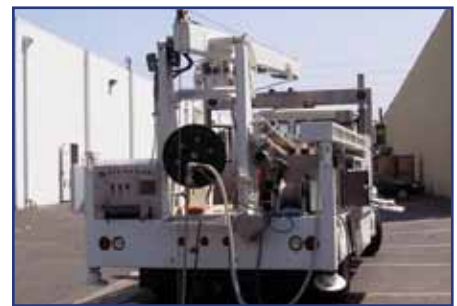
Pump/Development rigs are equipped with low clearance shieve blocks
