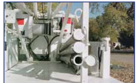
Self contained pump/development rig features an on-board steam cleaner and discharge pipe decontamination tubes
